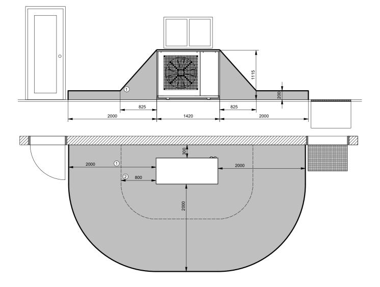
Fig. 6.4:Safety zone (floor level installation) around the heat pump
