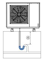
Fig. 6.8:Condensate pipe in channel over siphon
