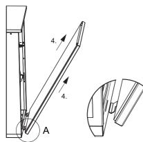
Fig. 7.4:Opening the side covering panels, work step 4
