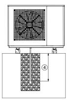
Fig. 6.7:Condensate drain in gravel
