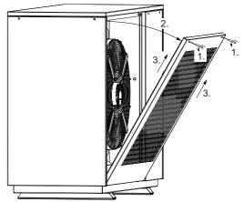
Fig. 7.1:Opening the grid panels
