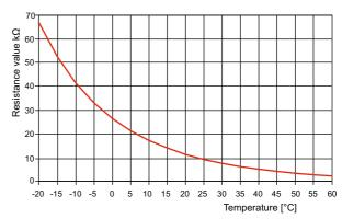
Fig. 7.8:Sensor characteristic curve NTC-10
