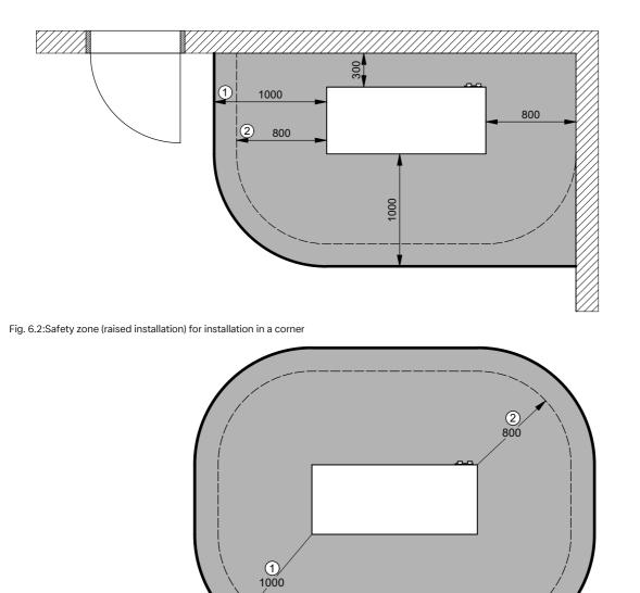
Fig. 6.3:Safety zone (raised installation) for installation in open space
