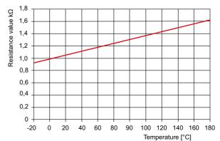
Fig. 7.10:Sensor characteristic curve PT 1000
