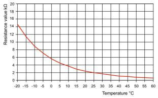
Fig. 7.9:Sensor characteristic curve NTC-2 according to DIN 50350 Outside temperature sensor
