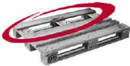
A board is missing
