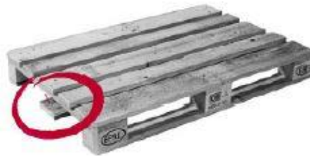
A block is missing or split to the point where more than one nail shank is visible.
