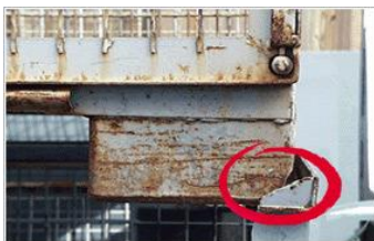
Bent base frame or feet
