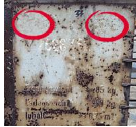
Possible contamination of the loaded goods due to large-scale rust/soiling
