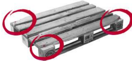
More than two lower or upper edge boards are damaged and more than one nail or screw shank is exposed
