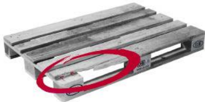
A single upper or lower edge board is damaged, so that more than one nail or screw shank is revealed.
