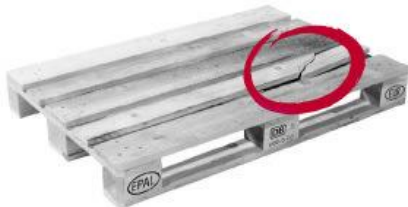
A board is broken transversely or diagonally
